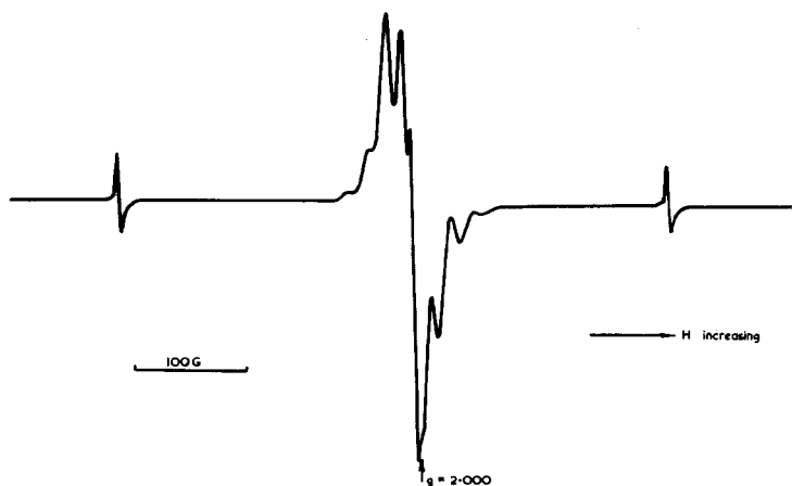
Figure 8 Full first derivative ESR spectrum from filed and \gamma -irradiated bovine bone, showing hydrogen lines. Sample prepared at 77 K spectrum recorded at 103 K.
